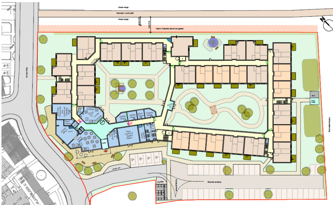
Layout of the ground floor entrance and communal areas (shown in blue) with the apartments shown surrounding the courtyard area.
